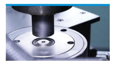
Graphite wound gaskets are manufactured of **Tensograph®** graphite foil by a special technology of Unichimtek similar to graphite rings production technology. This type of gaskets is highly efficient for sealing of 'tongue-groove' flanges and shaft connection to ball and gate in valve.
